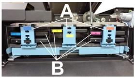
5. Close Ink Tank Door. Ink colors fill in as Ink Tanks are installed. If ink colors do not fill in after a few seconds, open Ink Tank Door again and reinstall Ink Tank(s).
